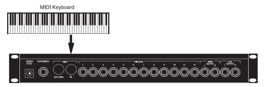
The [MIDI OUT/THRU] connector sends MIDI data from the DM5's keyboard to other MIDI devices, but can also send *System Exclusive* data (see the MIDI supplement in Appendix B) to a storage device for later recall. You can also convert the signals generated by the external triggers into MIDI signals to send out to other MIDI devices (such as a sequencer).
